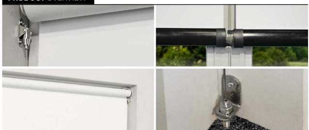
The Wire Guide System is designed to limit the free movement of the base rail of a roller blind that might cause damage or knocking against window recesses or glass. Wire guides are normally installed into areas with long drop blinds or areas exposed to high winds or draughts, such as from building A/C vents. The base rail is fitted with special end caps that encapsulate a fixed vertical wire that restrains the base rail from lateral movement.
