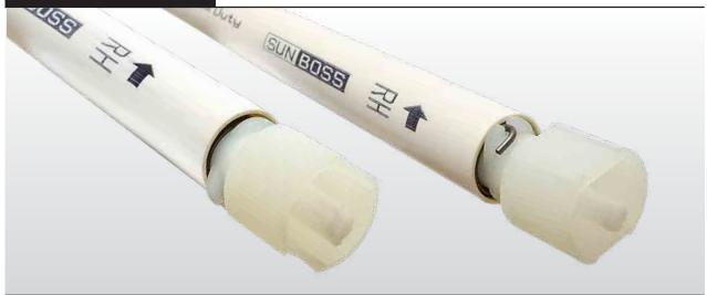
The **SunBoss** Standard Spring Assist is available in Light, Medium and Heavy-duty versions, all produced in LH and RH mounting configurations. The spring assist is designed to be compatible with all **SunBoss** 38mm clutches, which have a common end design that directly attaches to the spring with a retaining screw.
