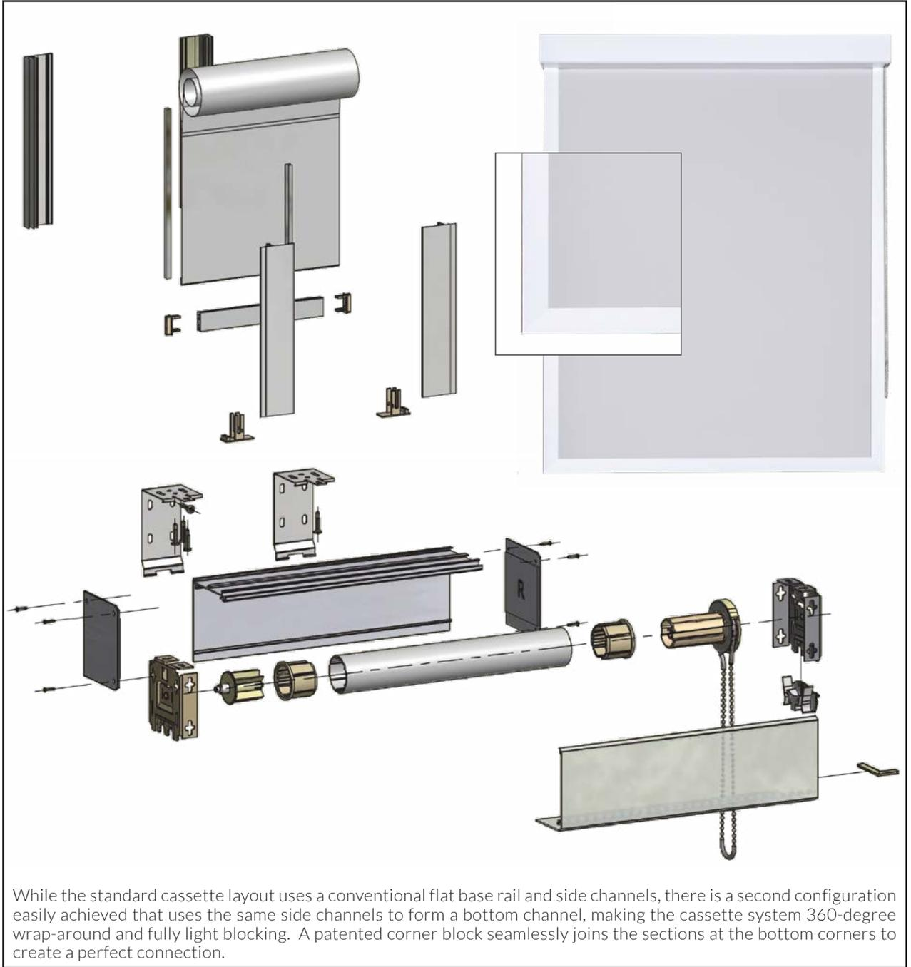
While the standard cassette layout uses a conventional flat base rail and side channels, there is a second configuration easily achieved that uses the same side channels to form a bottom channel, making the cassette system 360-degree wrap-around and fully light blocking. A patented corner block seamlessly joins the sections at the bottom corners to create a perfect connection.
